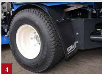
4 Fenders are equipped with a spatter guard made from rubber. The flexible material protect the machine from spatters of dirt and soil.
