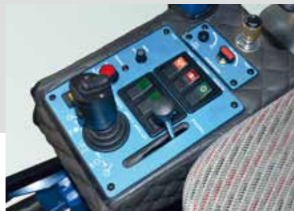
All buttons are placed close to the joystick – easy to reach.
