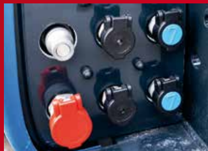
All VITRA machines are prepared for various attachments when delivered ( picture left: hydraulic couplings on the rear, Picture right: Hydraulic couplings in front)
