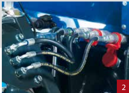
2 Flat face and leak free hydraulic couplings
