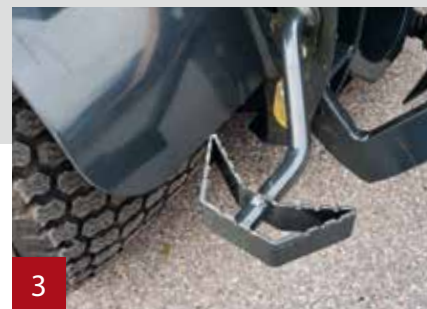
Door step placed under the cabin to ease the entry to the cabin.
