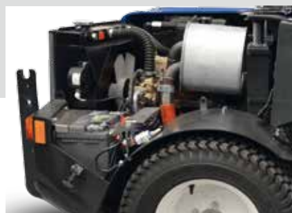
The Diesel tank turns away from the vehicle leaving space for service duties.
