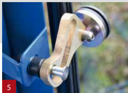
5 Windows are equipped with a hasp to increase the airflow in the cabin if needed.
