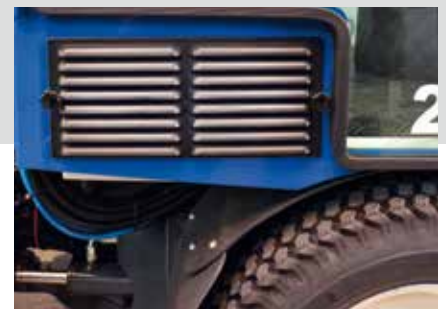
Air is cleaned through a filter before entering the cabin ventilation system – option is a pollen filter.
