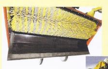
• The large debris container in the MultiSweep can be manually or hydraulically opened from within the carrier vehicle.
